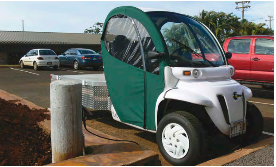
▲ Parked beside its own electric charging portal fed by the rooftop PV system, this GEM (Global Electric Motor) vehicle has zero emissions.
